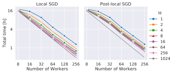
Figure 2: Total time in hours as a function of the number of workers for local SGD and post-local SGD. We report median time over 10 separate runs.
