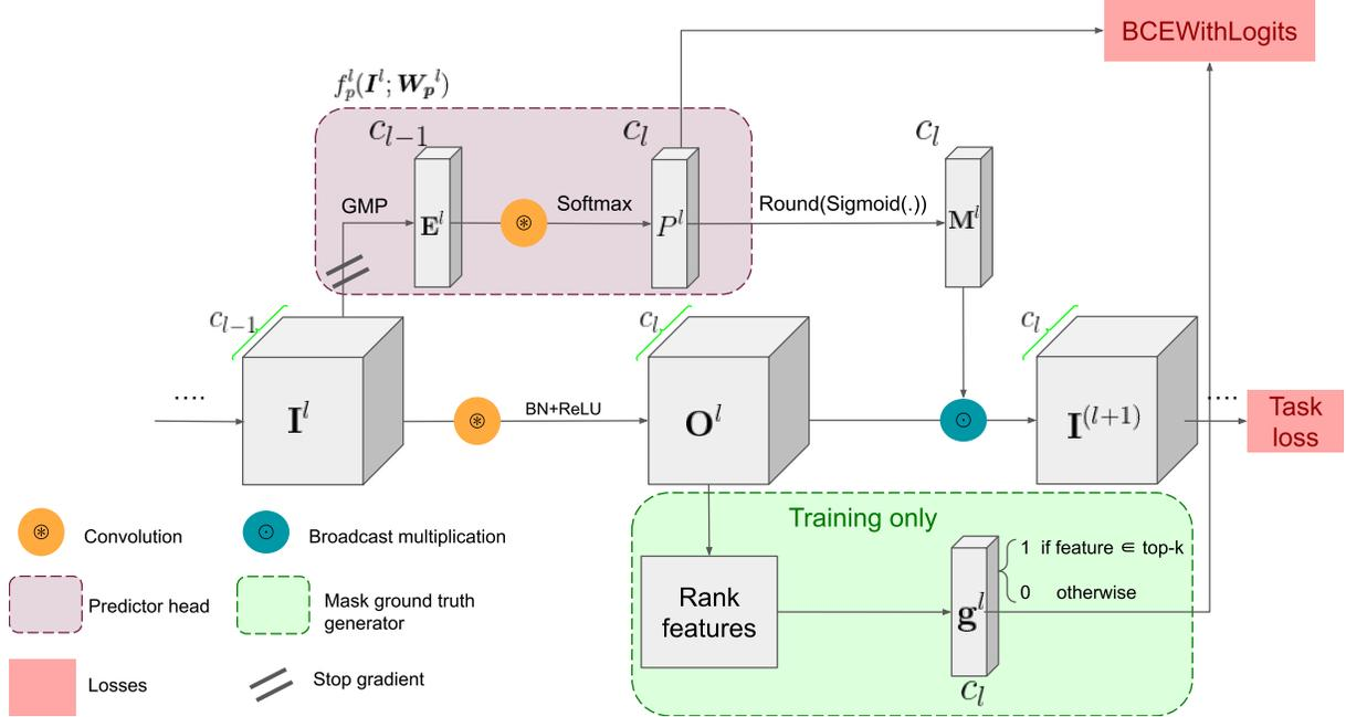
Figure 3. Proposed pipeline for training dynamic routing for one layer. For a layer  $l$ , prediction head  $f_p^l(I^l; W_p^l)$  takes an input  $I^l$ , applies global max pooling (GMP), normalizes with Softmax, then feeds to  $1 \times 1$  convolution to generate logits  $P^l$  for the binary mask  $M^l$ . Binary Cross Entropy (BCEWithLogits) loss penalizes the mask prediction based on the top- $k$  obtained from the unpruned feature maps  $O^l$ .
