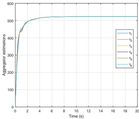
Fig. 7. Aggregator estimation of six generator systems.
