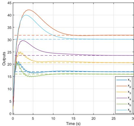
Fig. 4. Outputs of double-integrator agents by (17).
