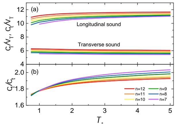
FIG. 1. Longitudinal ( $c_l$ ) and transverse ( $c_t$ ) sound velocities of generalized LJ  $n$ -6 fluids at freezing vs the reduced temperature  $T_*$ . In (a) sound velocities are expressed in units of the thermal velocity  $v_T$ ; Upper curves are for the longitudinal mode, lower curves are for the transverse mode. In (b) the ratio of the longitudinal-to-transverse sound velocities,  $c_l/c_t$  is plotted.
