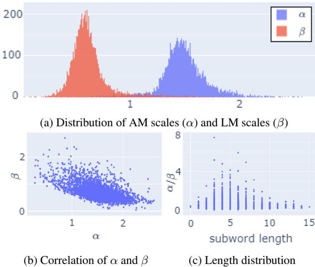
**Fig. 1:** Analysis of subword dependent AM scales  $\alpha$  and LM scales  $\beta$  trained on LibriSpeech 960h with minWER criterion
