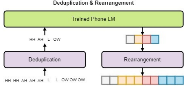
Fig. 2. Deduplication: Several consecutive overlapping labels are distributed in the forced alignment generated through the Gaussian Mixture-Hidden Markov Model-based speech recognition system (GMM-HMM-based ASR). We remove the overlapped labels through the deduplication algorithm (this algorithm also includes matching the units of forced alignment and LM outputs). Rearrangement: The rearrangement algorithm aligns the list of posterior distributions of the LM one-to-one with the forced alignment before the deduplication process.
