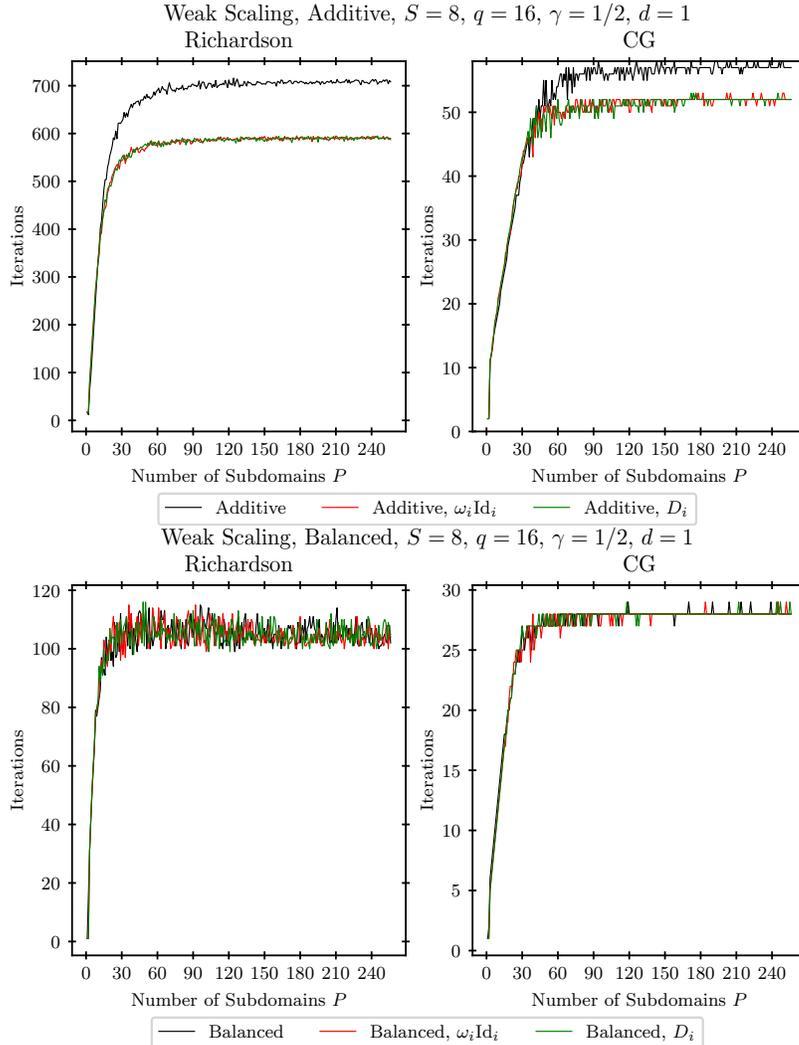
Figure 4: Weak scaling: Number of iterations  $K$  versus number of subdomains for the linear/Richardson iteration (left) and the associated preconditioned conjugate gradient method (right), preconditioned by the three differently weighted versions of the *additive* (top) and the *balanced* (bottom) scheme,  $d = 1$ ,  $q = 16$ ,  $\gamma = 0.5$ .
