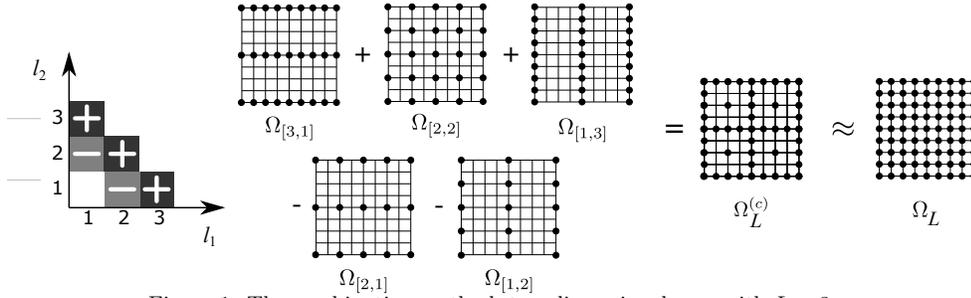
Figure 1: The combination method, two-dimensional case with  $L = 3$ .
