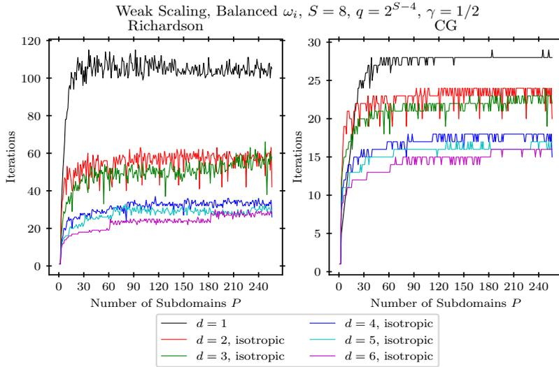
Figure 8: Weak scaling: Number of iterations versus number of subdomains for the  $\omega_i$ -weighted balanced linear/Richardson iteration (left) and the associated preconditioned conjugate gradient method (right) for different dimensions  $d$ ,  $q = 2^{S-4}$ ,  $\gamma = 0.5$ .
