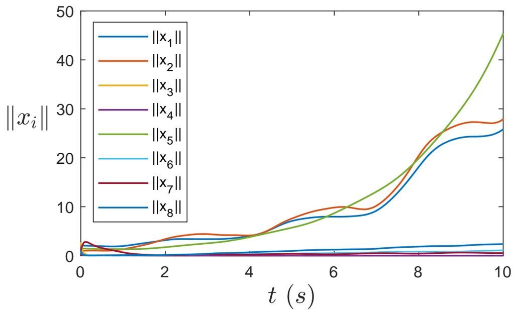
Fig. 2: Compromised system: Divergent trajectories show that a smart attacker, with limited resources, can easily compromise a fixed (predictable) control sublayer 1.
