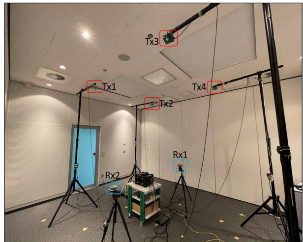
Fig. 1. Measurement scenario in an empty conference room. Transmitters and receivers are marked in red and blue color.
