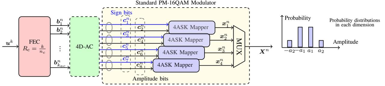
Fig. 1. Signal shaping via four-dimensional amplitude coding (4D-AC). An example of probability distribution for each 1D is shown at the output of modulator.
