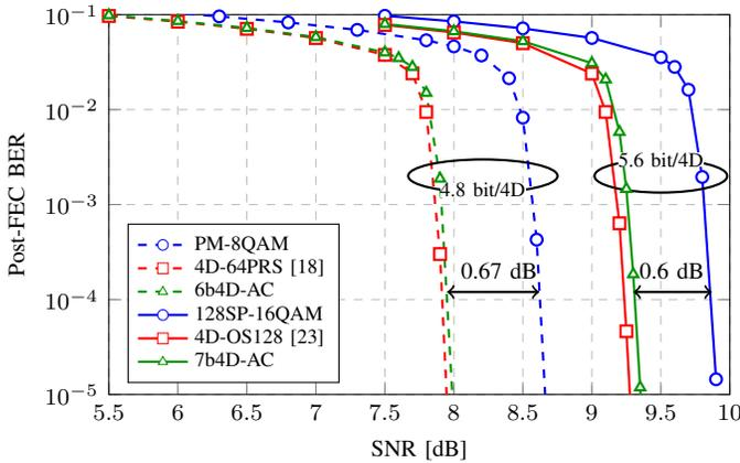
Fig. 5. BER vs. SNR for different modulation formats at transmission rates of 4.8 bit/4D-sym and 5.6 bit/4D-sym, respectively. Rate- $R_c = 0.8$  DVB-S2 LDPC codes of length  $n_c = 64800$  bits are used.
