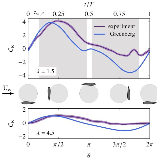
Figure 3: Comparison between the experimentally obtained phase-averaged radial force coefficient and the prediction based on the modified Greenberg model for (top)  $\lambda = 1.5$  and (bottom)  $\lambda = 4.5$ . The shaded areas in correspond to regions where the magnitude of the effective angle of attack is above the critical stall angle.
