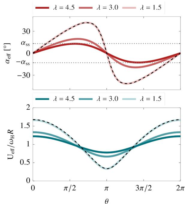
Figure 2: Temporal evolution of the a) effective angle of attack and b) effective flow velocity over a single rotation of a vertical-axis wind turbine blade for  $\lambda \in \{1.5, 3.0, 4.5\}$ . The dashed line represents the Fourier series approximation for  $\lambda = 1.5$  Horizontal dotted lines indicate the static stall angle for a NACA0018 airfoil ( $\alpha_{ss} = 13.1^\circ$  at  $Re = 50\,000$ ).
