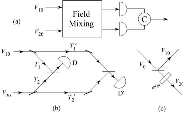
FIG. 1. (a) General scheme of fourth-order interference between two fields by field mixing. (b) A specific scheme of field mixing by using beam splitters. (c) Generation of two fields with a random phase  $\varphi$  from one field by a beam splitter.
