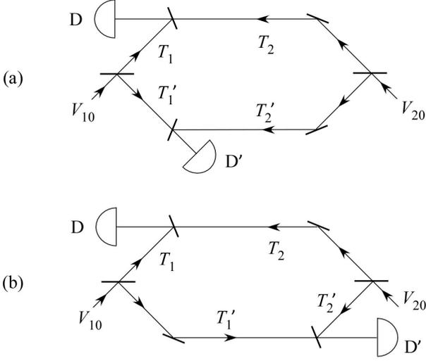
FIG. 3. Schemes of fourth-order interference between two fields with (a)  $T_1 \sim T_1'$  and  $T_2 \sim T_2'$ , but  $|(T_1, T_1') - (T_2, T_2')| \gg T_c, T_R$  (Scenario (ii)); (b)  $T_1 \sim T_2'$  and  $T_2 \sim T_1'$ , but  $|(T_1, T_2') - (T_2, T_1')| \gg T_c, T_R$  (Scenario (iii)).
