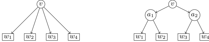
Fig. 7. A general DAG can be replaced by a new binary DAG obtained by adding auxiliary nodes, which corresponds to the same game.
