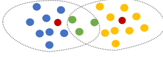
Figure 4: Closure clustering assignment: assign boundary vectors (green points) to multiple closest clusters if its distances to these clusters are nearly the same (blue and yellow clusters).
