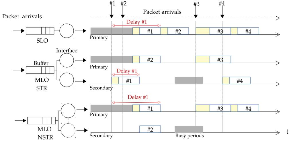
Fig. 1: Illustration of SLO, MLO-STR, and MLO-NSTR operations. Grey, yellow, and white bars respectively indicate occupied channels, random backoffs, and packet transmissions. Packet transmissions include both the data part and the corresponding ACK, as well as DIFS and SIFS inter-frame spaces.
