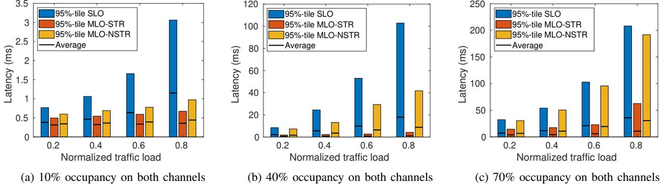
Fig. 3: Latency for symmetrically occupied channels vs. variable normalized traffic load.
