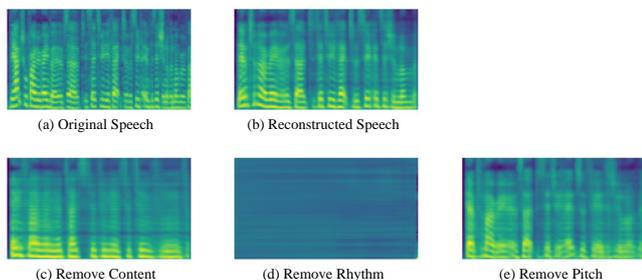
Fig. 2. The spectrogram reconstructed by SpeechFlow. The model was trained with VCTK, and the speech signal was selected from IEMOCAP. (a) spectrogram of the original speech; (b) spectrogram of the reconstructed speech with all the information factors preserved; (c)~(e) spectrograms of the reconstructed speech with a single information factor removed.
