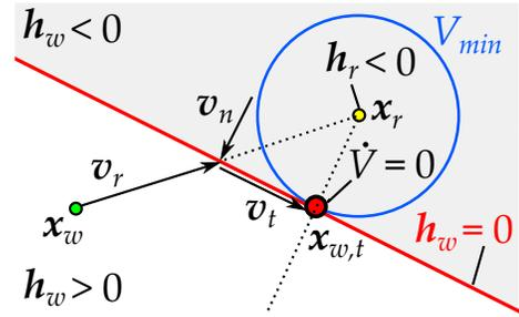
Fig. 3. Explicit Reference Governor (ERG) manipulates the applied reference states  $\mathbf{x}_w$  to be as close as possible to the desired reference  $\mathbf{x}_r$  without violating the constraint equation  $\mathbf{h}_w \geq 0$ .
