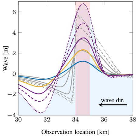
**Figure 5.** Comparison of waves on shore modeled by the shallow water equations and their linearization about the rest state. The waves are initialized by the bathymetry change corresponding to the optimizers from Figure 4. Snapshots show the waves when their average is largest in the observation interval. The gray waves, shown for reference, are the same as in Figure 4(C). The waves shown in color are obtained by solving the linearized equations using the same initializations.
