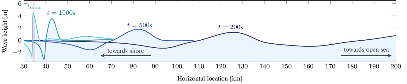
**Figure 1.** Snapshots of tsunami waves generated by the optimizer with  $z = 4$  (dashed line in Figure 4B) at different times  $t$ . The seafloor deformation generates waves in both directions, but we focus on the waves traveling towards the shore on the left. The region where we measure average tsunami height at time  $t_{\max}$  is shaded in red. Note that the tsunami wave is compressed as it travels towards shore, its magnitude increases and its leading wave edge steepens.
