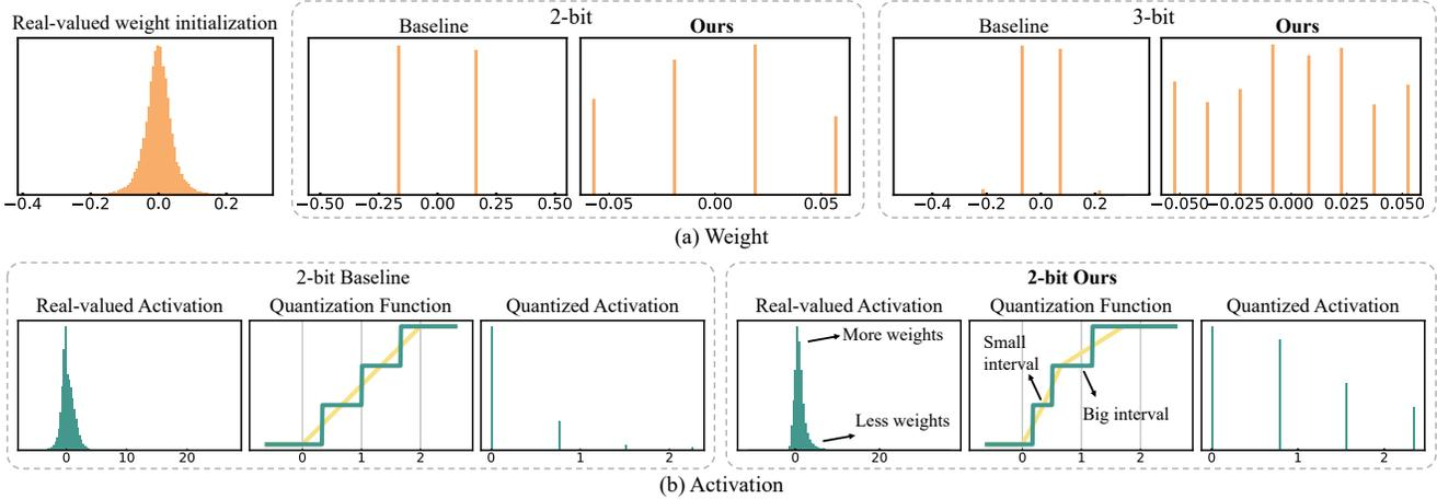
Figure 3. Histogram of the weight and activation distribution.
