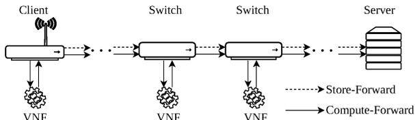
Fig. 2: Overview of the in-network data processing scenario.
