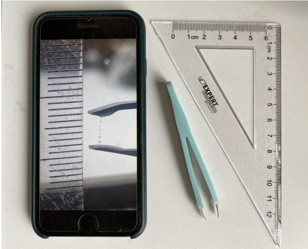
Fig. 2. Experimental equipment for studying the rheology of elastic fluids: a smartphone, tweezers and a ruler
