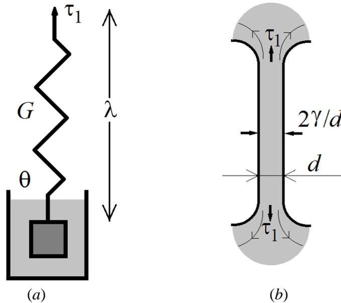
Fig. 5. Models of viscoelastic rheology (*a*) and thinning filament (*b*)
