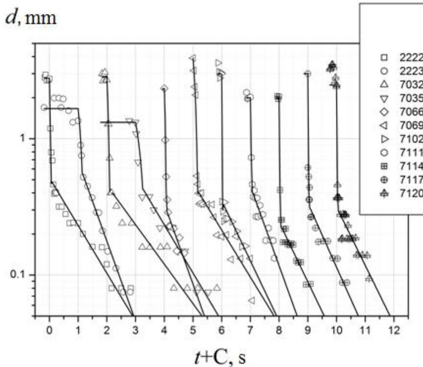
Fig. 6. Dependences of the filament diameters versus time according to the data of 8 experiments (symbols and numbers of experiments are shown in the inset). For clarity, the curves are shifted in time with a step of 1 s. The horizontal lines in some curves show the droplet size before the start of stretching. Solid piecewise linear dependences are the fittings of experimental points by analytical dependence (6)
