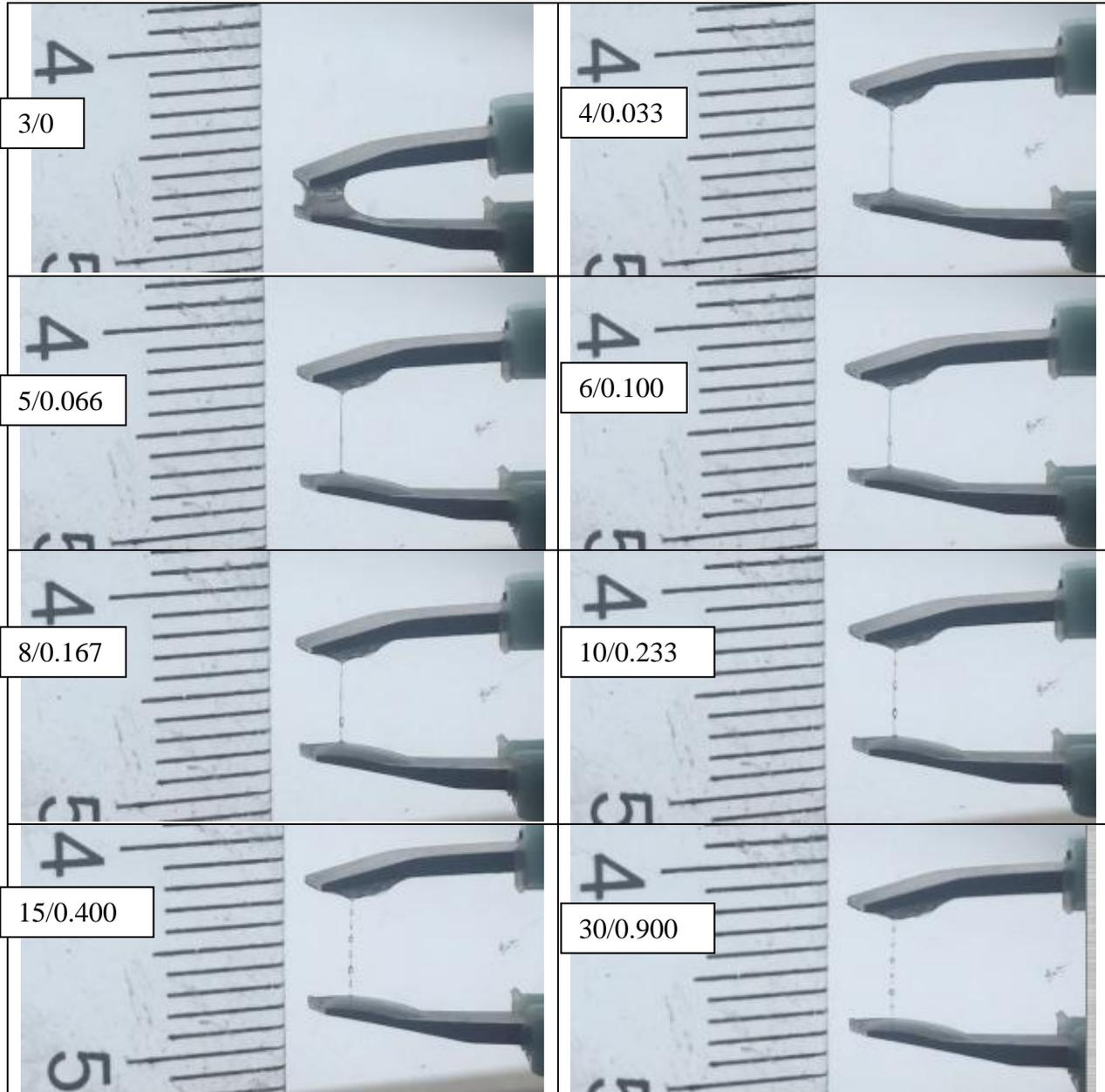
Fig. 3. Video recording of the formation and thinning of the oral fluid filament (experiment 7114, also see Figs. 4, 5). Time increases from left to right and from top to bottom. The insets indicate the frame number / filament thinning time (seconds)
