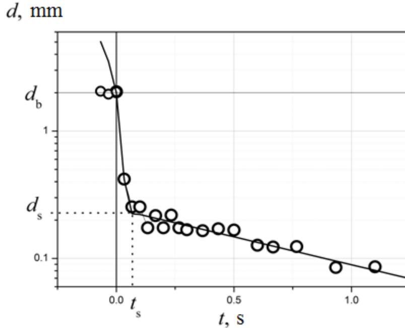
Fig. 4. Thinning of the filament of the oral fluid – dependence of the filament diameter as function of time. Solid curve – fitting of experimental points (experiment 7114) by analytical dependence (6) for points  $t > 0$
