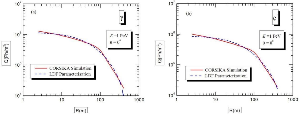
**Figure 1.** Lateral distribution of Cherenkov light which simulated with CORSIKA code (solid lines) and one parameterized (Eq. (3)) (symbol lines) at 1 PeV for vertical showers initiated (a) by primary gamma quanta; (b) by primary electron.
