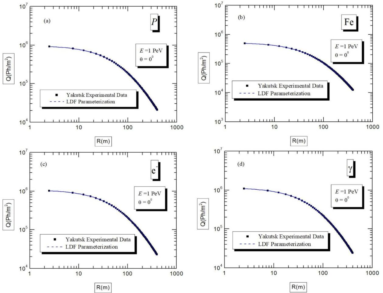
**Figure 3.** Comparison of the parameterized Cherenkov light LDF (Eq. (3)) with the data obtained by the Yakutsk EAS array (symbols) for vertical showers of (a) primary proton; (b) iron nuclei; (c) primary electron; (d) gamma quanta.
