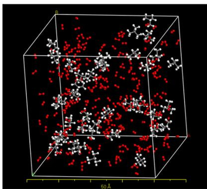
Fig. 1 Simulation box of iso-butane
