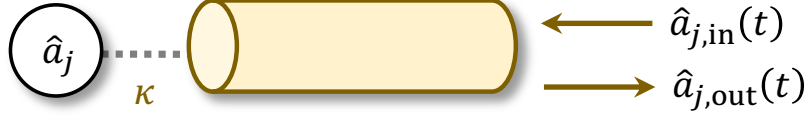
Figure 2: Schematic showing a single cavity (lowering operator \hat{a}_j ) coupled to an input-output waveguide or transmission line. \hat{a}_{j,\text{in}} encodes the the amplitude of signals and noise incident on the cavity, whereas \hat{a}_{j,\text{out}} encodes the amplitude of signals and noise leaving the cavity.
