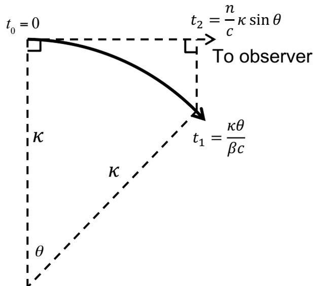
FIG. 6. Sketch of the time delays associated with synchrotron radiation. At time  $t_0 = 0$  a particle is oriented towards an observer. After subtending an angle  $\theta$  with curvature radius  $\kappa$  at velocity  $v = \beta c$ , it is time  $t_1 = \kappa \theta (\beta c)^{-1}$ . Radiation emitted at time  $t_0$  takes a time  $t_2 = (n/c) \kappa \sin \theta$  to be equidistant to the observer.
