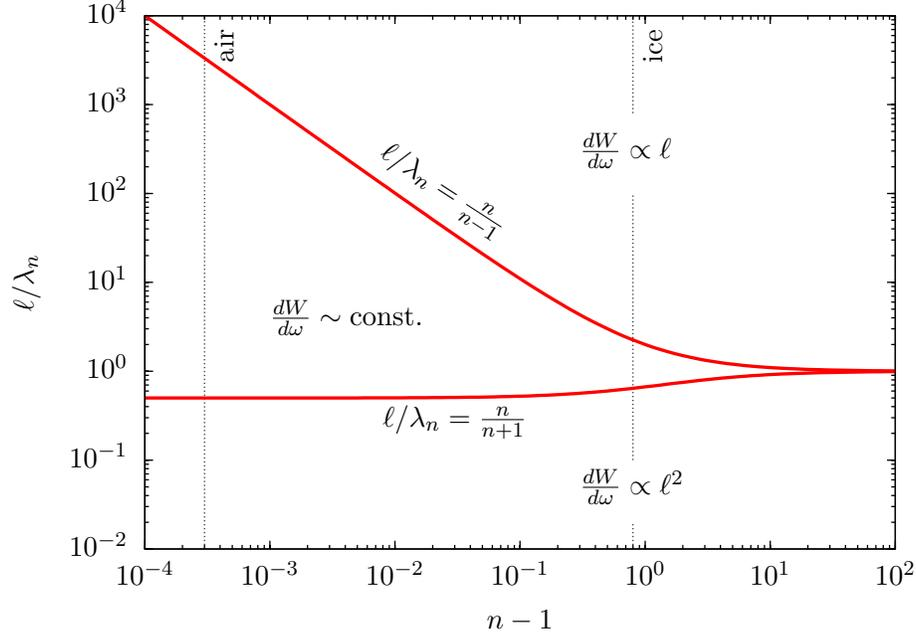
FIG. 4. Illustration of the regimes in track-length  $\ell$  and medium refractive index  $n$  over which the emitted radiation will appear Cherenkov-like (radiated power  $dW/d\omega \propto \ell$ ), bremsstrahlung-like ( $dW/d\omega$  constant), or as an unresolved point-source ( $dW/d\omega \propto \ell^2$ ). The values of  $n - 1$  for air and ice applicable to radio wavelengths are also indicated as vertical lines.
