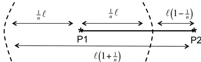
FIG. 1. Sketch of the electromagnetic shock front (dotted line) from a particle initially accelerated at P1 in a medium with refractive index  $n$  and having travelled a distance  $\ell$  to P2 with uniform velocity  $\beta = 1$  (solid line).
