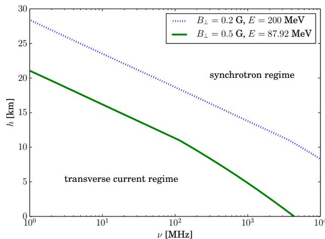
FIG. 8. Height  $h$  in the atmosphere at which  $\ell_{\text{synch}} = \chi_0$ , computed for two combinations of magnetic field / electron energy. Above this height is the synchrotron regime where  $\ell_{\text{synch}} < \chi_0$ , and below this the transverse-current regime, where  $\ell_{\text{synch}} > \chi_0$ .
