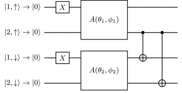
FIG. 1: Ansatz circuit used to represent the ground state of the two-site Fermi-Hubbard model with two electrons in the VQE scheme. The particle-number conserving  $A$  gates are those defined in Eq. (18). The  $X$  gates set the correct values for the number of particles and the spin projection  $S_z$ . The overall circuit then conserves these quantities.
