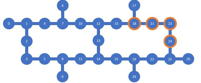
FIG. 2: Picture of the topology of the *ibm\_cairo* 27 qubit device. We highlight in orange the qubits used to implement our algorithm.
