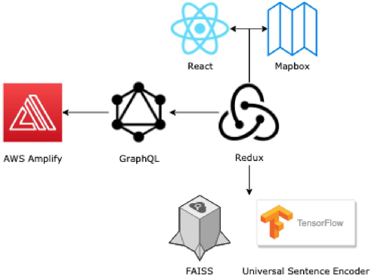
Figure 3: Projection Architecture
