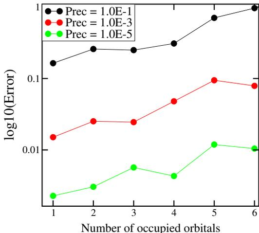
FIG. 2. Error as a function of the number of occupied states for a single water molecule with  $N = 6$ . Results for three different precision values are shown.
