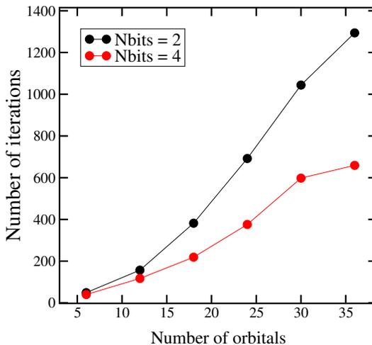
FIG. 4. Number of iterations as a function of the system size (number of orbitals). Calculations using two and four bits of precision are shown.
