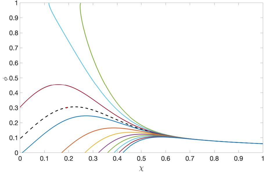
FIG. 8. Curves  $(\chi(\tau), \phi(\tau))$  for  $P = 32$  and (solid curves)  $0.64102 \leq F \leq 0.64103$  in increments of  $10^{-6}$ , with  $F$  increasing from the top curve to the bottom curve. Initially  $(\chi(0), \phi(0)) = (1, 0.06)$  and  $\tau$  increases from right to left. The red dot shows the desired geometry  $(\chi_T, \phi_T) \approx (0.1911, 0.3)$  at the tip  $x = 0$ . The black-dashed curve passing through the red dot corresponds to a force of  $F = 0.64102262$ .
