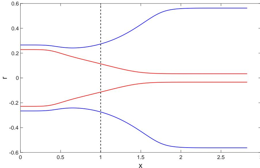
FIG. 4. The outer boundary  $r = R(x,t)$  (blue) and inner boundary  $r = \phi(x,t)R(x,t)$  (red) over the position after pulling from an initial length of  $L(O) = 1.5$ , cross-sectional area  $\chi^2(x,0) = 1$ , and aspect ratio  $\phi(x,0) = 0.06$  for an internal channel pressure  $P = 34.217$ , force  $F = 1.32$ , and a draw time  $t_K = 0.44$ .
