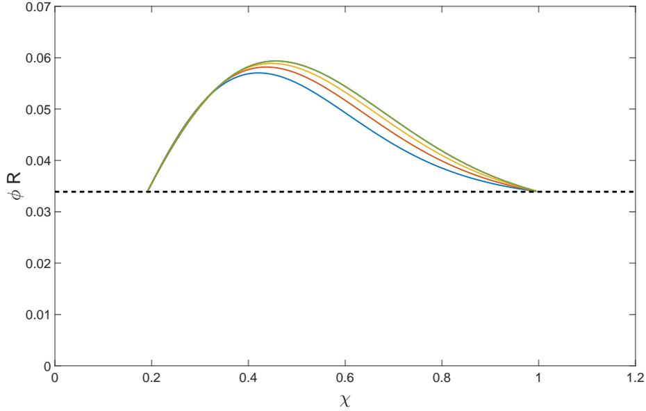
FIG. 6. Plot of the internal boundary  $r = \phi R$  as a function of  $\chi \in [\chi_T, 1]$  for (bottom to top)  $P = 34, 35, 36, 37$  and corresponding  $F = 1.3166, 1.5597, 1.7730, 1.9690$ , respectively (to four decimal places), for a tube with initial aspect ratio  $\phi_0 = 0.06$ . The black dashed line shows the initial inner radius (when  $\chi = 1$ ) which is also the radius when  $\chi = \chi_T = 0.1911$ .
