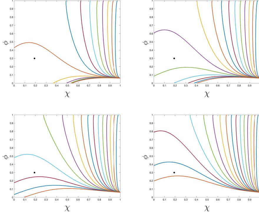
FIG. 5.  $\phi$  versus  $\chi$  for a capillary with initial aspect ratio  $\phi_0 = 0.06$ . Pulling with pressure  $P = 34$  (top left), 35 (top right), 36 (bottom left), 37 (bottom right) for a force  $F$  ranging from 0.5 to 2 in increments of 0.1. The black dot is  $(\chi_T, \phi_T) = (0.1911, 0.3)$  corresponding to the final emitter geometry at  $x = 0$ .
