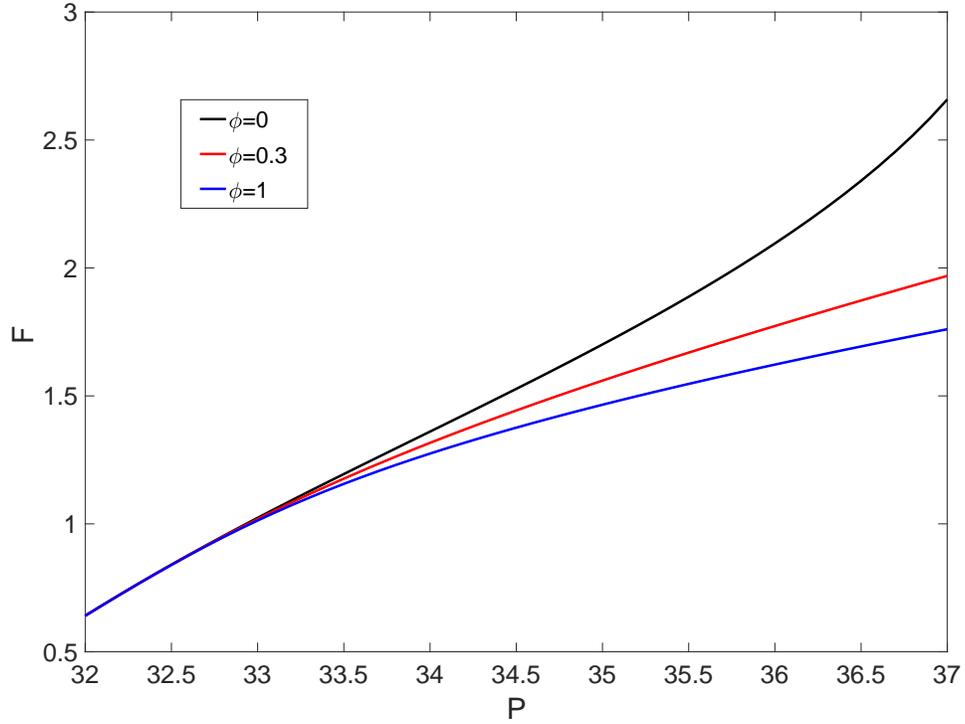
FIG. 9. Pulling force  $F$  versus pressure  $P$  for the manufacture of emitters with  $\chi_T = 0.1911$  and  $\phi_T = 0$  (black),  $\phi_T = 0.3$  (red) and  $\phi_T = 1$  (blue), from a tube with initial geometry  $(\chi, \phi) = (1, 0.06)$ .
