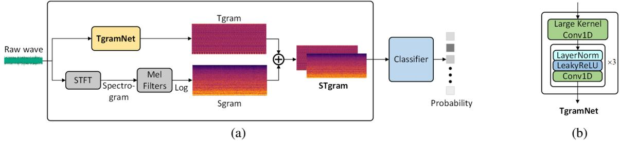
**Fig. 1.** The framework of the proposed method for anomalous sound detection. (a) The spectral-temporal feature is extracted from the raw wave through a CNN-based network (TgramNet) for the temporal feature and the log-Mel spectrogram for the frequency feature.  $\oplus$  denotes concatenation operation for feature fusion. The spectral-temporal feature is then fed into the classifier for anomalous sound detection. (b) Details in TgramNet.
