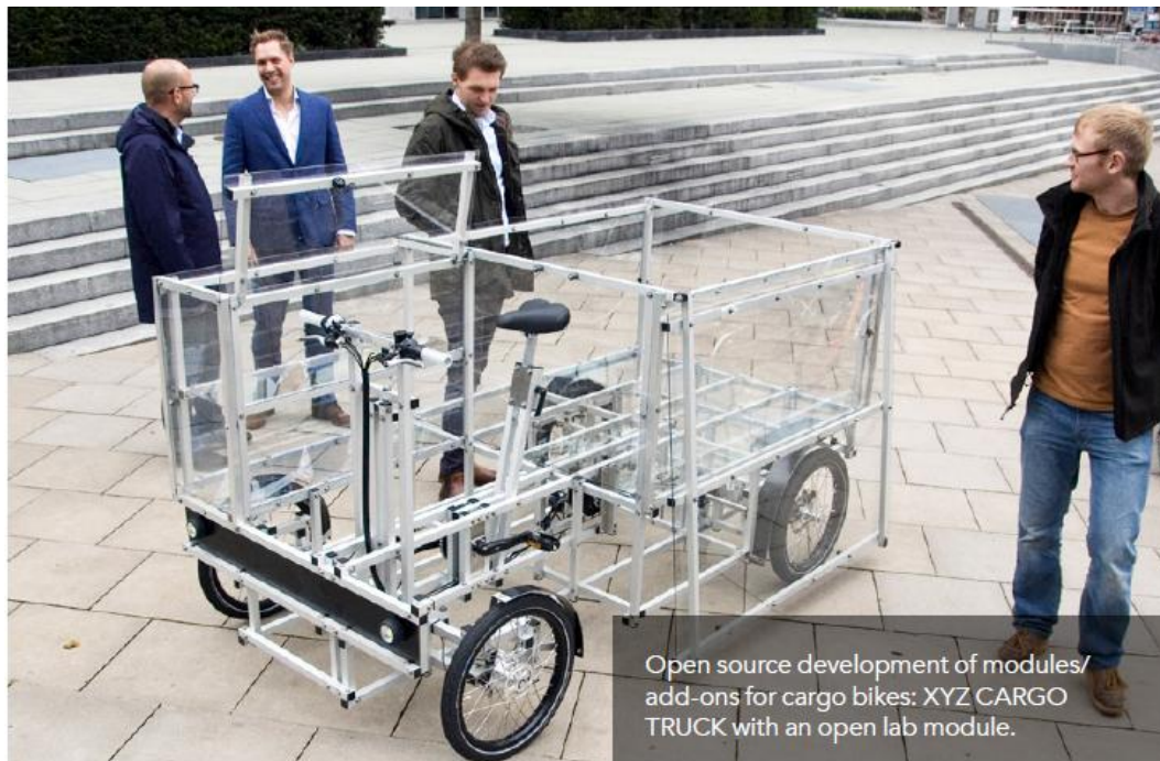
Figure 10: Open source development of modules/add-ons for cargo bikes: XYZ CARGO TRUCK with an open lab module [64]
