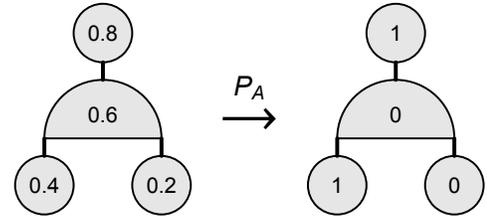
FIG. 3. Logic assignment projection,  $P_A$ , applied to a gate (semicircle) taking two inputs. The gate may have two states:  $f = 0$  for OR and  $f = 1$  for AND.
