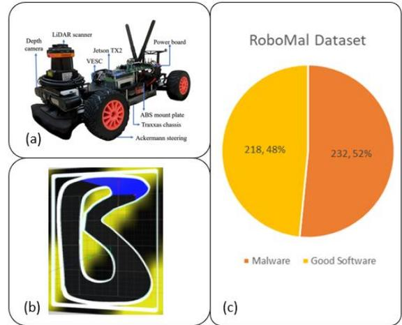
Fig. 1: The RoboMal Dataset; (a) The F1/10 autonomous car with multiple sensors [23], (b) The wall follower track in Gazebo simulator, and (c) The distribution of malware and good software in RoboMal dataset.
