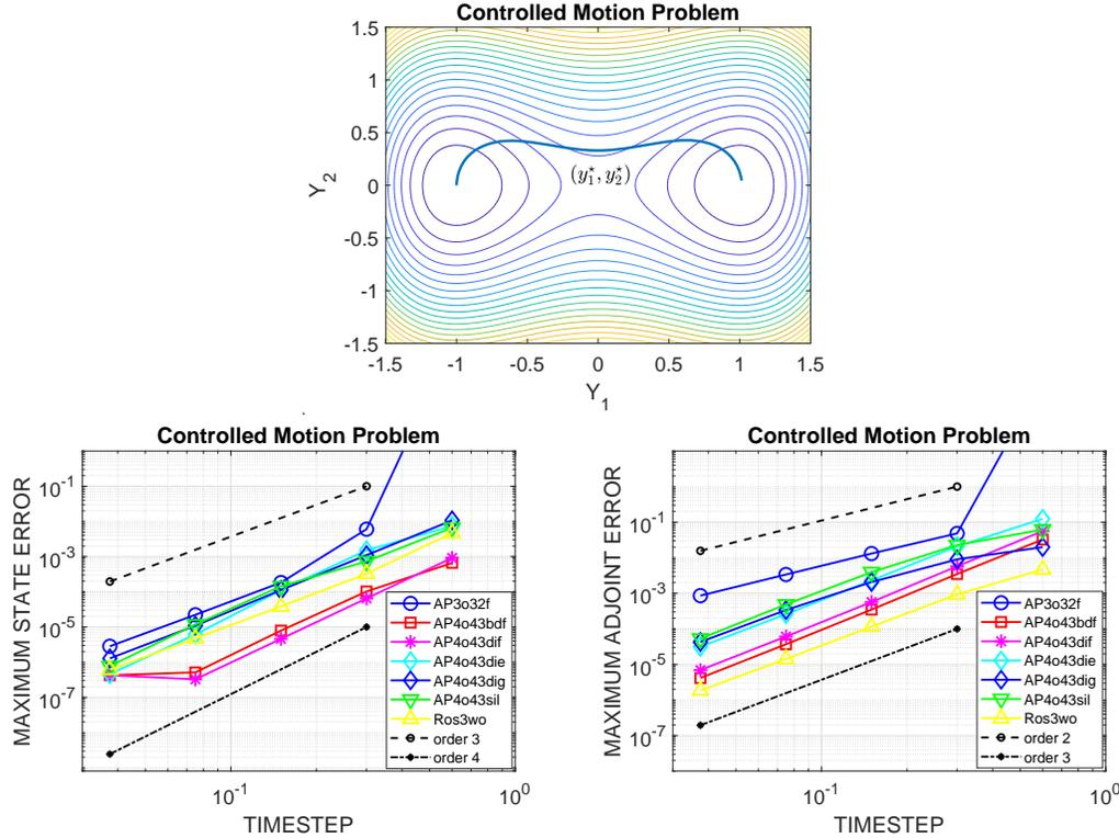
Figure 2: Controlled Motion Problem: optimal path  $(y_1^*, y_2^*)$  through the total energy field  $E = \frac{1}{2}y_2^2 + \frac{1}{4}y_1^4 - \frac{1}{2}y_1^2$  visualized by isolines and exhibiting a saddle point structure (top). Convergence of the maximal state errors  $\|(w^T \otimes I)Y_n - y(t_{n+1})\|_\infty$  (bottom left) and adjoint errors  $\|(v^T \otimes I)P_n - p(t_n)\|_\infty$  (bottom right),  $n = 0, \dots, N$ .
