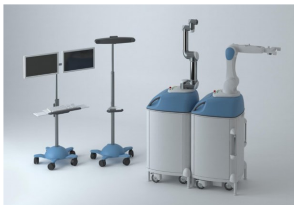
Fig. 2. The 3 rd generation of the robotic system RONNA with an assistant (left) and master robot (right)
