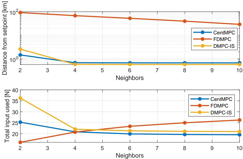
**Fig. 3** Relative position error averaged for all the simulations in the top plot, with the y-axis in log scale, and total input averaged for all the simulations in the bottom plot.
