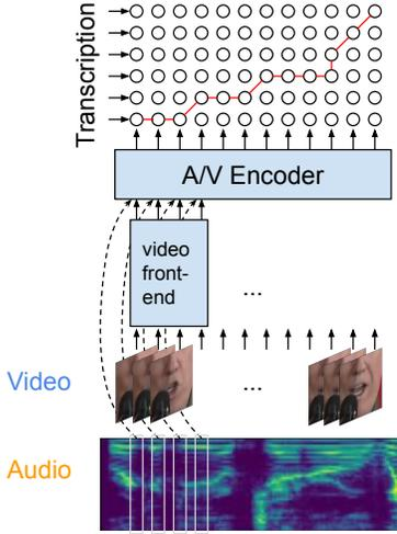
**Fig. 1.** An overview of end-to-end AV-ASR and lip reading models. The video is encoded with a video front-end. The visual features and the acoustic features are concatenated and fed through the AV encoder to be used for the RNN-T loss.
