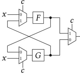
Fig. 4. An example of a cyclic combinational circuit, adapted from [32, Fig. 1], where  $F$  and  $G$  are arbitrary combinational circuits.
