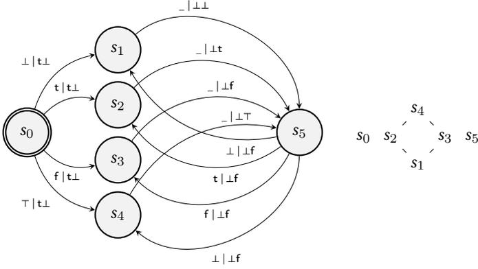
Fig. 6. On the left, the Mealy machine from Example 53, where a transition label  $v|w$  indicates an input  $v$  and an output  $w$ . On the right, the corresponding state ordering.
