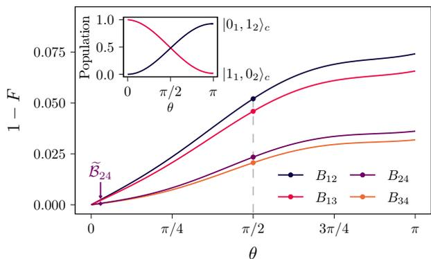
FIG. 3. Beam-splitting transformation between motional modes. The detunings are set to  $\delta_1 = \nu_j - \nu_k$  and  $\delta_2 = -(\nu_j - \nu_k)$  for the transformation (34). Main plot: infidelity against angle of rotation  $\theta$ , acting on pairs of collective modes. Inset: population of states  $|0_1, 1_2\rangle_c$  and  $|1_1, 0_2\rangle_c$  for the same range of  $\theta$ .
