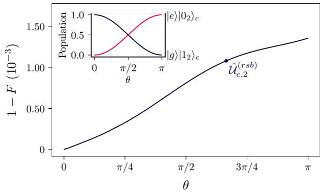
FIG. 2. Red sideband transition. Main plot: infidelity of the target state against the angle of rotation,  $\theta$ , acting on the 2<sup>nd</sup> collective mode. Inset: population of the states  $|e\rangle|0_2\rangle_c$  and  $|g\rangle|1_2\rangle_c$  for the same range of  $\theta$ .
