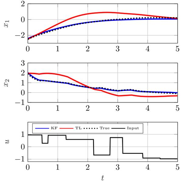
Fig. 2. Open loop prediction of KoopmanizingFlows (KF) compared to Taylor linearization around equilibrium (TL) for the Example 1
