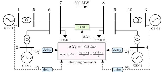
Fig. 5. Schematic of 4-machine system with damping controller
