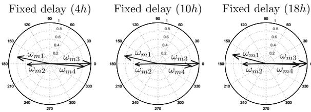
Fig. 7. Inter-area swing mode eigenvector: generator speed components
