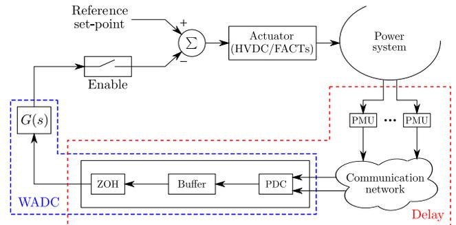
Fig. 1. Schematic of a power system with a WADC
