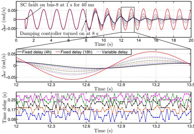
Fig. 8. Time-domain simulations of the system with variable delay
