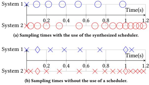
**Figure 8: Sampling times of the first 1.2 seconds of the simulation in Figure 7. For reference, the sampling times when no scheduler is used are shown in (b). Early triggers are denoted with a 'o'. Sampling collisions are represented with a 'x'.**
