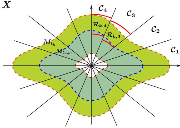
**Figure 1: IM-based partitioning for a homogeneous CETC system.** The rays passing through the origin determine the cones  $C_j$ . The dashed lines are consecutive approximations of IMs  $M_{t_k}$  and  $M_{t_{k+1}}$ . The regions  $\mathcal{R}_{k,j}$  are delimited by consecutive approximations of IMs and cones (hence the indexing). The circular segments in cones  $C_3$  and  $C_4$  delimit the ball segments that overapproximate regions  $\mathcal{R}_{k,3}$  and  $\mathcal{R}_{k,4}$ .
