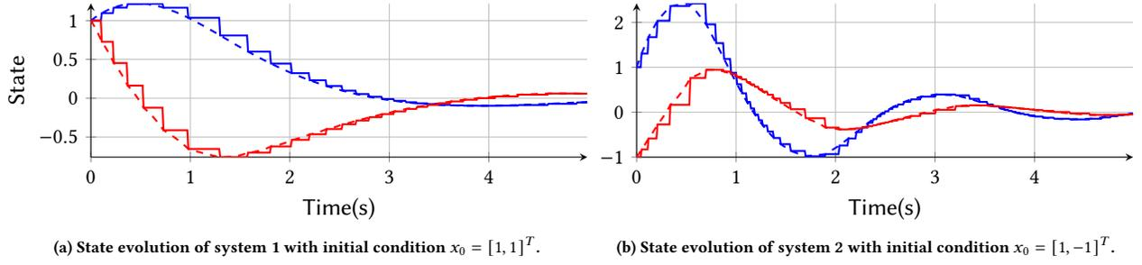
**Figure 7: Evolution of the systems' states under the scheduler synthesized as detailed in Section 4.4. Dashed lines represent the actual state evolution, while the solid lines represent the states available to the controller at each time.**
