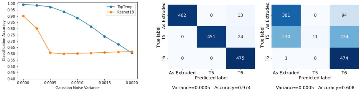
Figure 2: The classification test accuracies for *TopTemp* and ResNet18 for different levels of Gaussian noise are shown in the leftmost plot. The confusion matrices for Gaussian noise variance 0.0005 are shown for *TopTemp* SSVm (middle) and the fine tuned ResNet18 model (right).
