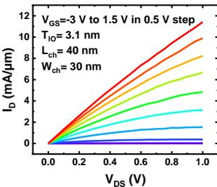
Fig. 12. Output characteristics of an  $\text{In}_2\text{O}_3$  GAA nanoribbon FET with  $W_{\text{ch}}$  of 30 nm, showing maximum  $I_{\text{ON}}$  of 11.4  $\text{mA}/\mu\text{m}$  at  $V_{\text{DS}} = 1 \text{ V}$ .
