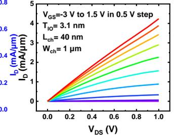
Fig. 7. Output characteristics of a typical  $\text{In}_2\text{O}_3$  GAA FET with  $L_{\text{ch}}$  of 40 nm and  $W_{\text{ch}}$  of 1  $\mu\text{m}$ , showing maximum  $I_{\text{ON}}$  of 4.3  $\text{mA}/\mu\text{m}$  at  $V_{\text{DS}} = 1 \text{ V}$ .
