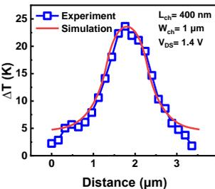
Fig. 13. Cross-sections of the experimental and simulated results of temperature increase  $\Delta T$  of an  $\text{In}_2\text{O}_3$  GAA nanoribbon FET with  $W_{\text{ch}}$  of 1  $\mu\text{m}$ .
