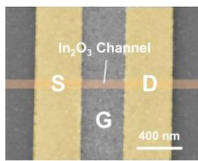
Fig. 9. False-color top-view SEM image of an  $\text{In}_2\text{O}_3$  GAA nanoribbon FET with  $W_{\text{ch}}$  of 50 nm.
