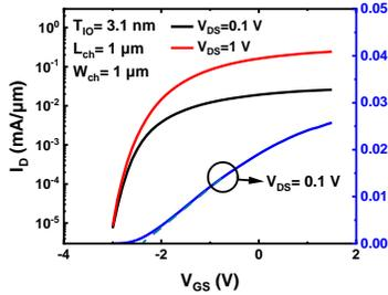
Fig. 4. Transfer characteristics of a typical  $\text{In}_2\text{O}_3$  GAA nanoribbon FET with  $L_{\text{ch}}$  of 1  $\mu\text{m}$  and  $W_{\text{ch}}$  of 1  $\mu\text{m}$ .
