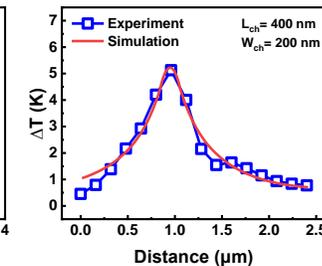
Fig. 14. The same TR measurements and simulations of a device with  $W_{\text{ch}}$  of 200 nm. Space resolution is limited to hundreds of nm for TR measurement.
