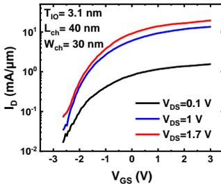
Fig. 16. Pulsed I-V results of transfer characteristics of an  $\text{In}_2\text{O}_3$  GAA FET with  $L_{\text{ch}}$  of 40 nm and  $W_{\text{ch}}$  of 30 nm.
