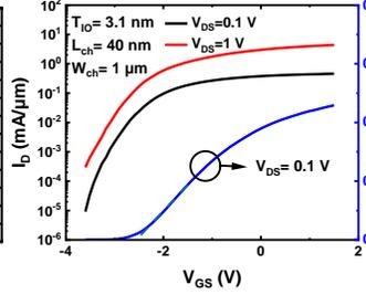
Fig. 6. Transfer characteristics of a typical  $\text{In}_2\text{O}_3$  GAA FET with  $L_{\text{ch}}$  of 40 nm and  $W_{\text{ch}}$  of 1  $\mu\text{m}$ .
