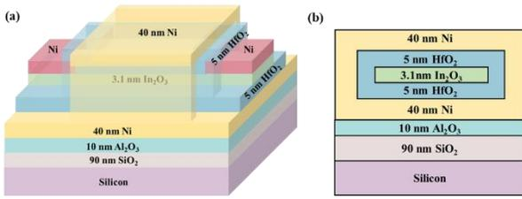
Fig. 1. Device schematic of an  $\text{In}_2\text{O}_3$  GAA nanoribbon FET with  $T_{\text{IO}}$  of 3.1 nm and dielectric of 5 nm  $\text{HfO}_2$  in (a) 3D model (b) cross-section view in S/D direction.
