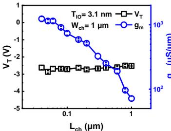
Fig. 8.  $V_{\text{T}}$  and  $g_{\text{m}}$  scaling metrics of  $\text{In}_2\text{O}_3$  GAA FETs with  $L_{\text{ch}}$  from 40 nm to 1  $\mu\text{m}$  and  $W_{\text{ch}}$  of 1  $\mu\text{m}$ .  $g_{\text{m}}$  is extracted at  $V_{\text{DS}} = 1 \text{ V}$ .
