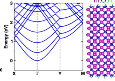
Fig. 18. DFT band structure of 3.0 nm thick  $\text{In}_2\text{O}_3$  slab, with the lowest conduction band having an effective mass of 0.19  $m_0$ .
