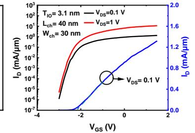
Fig. 11. Transfer characteristics of a typical  $\text{In}_2\text{O}_3$  GAA nanoribbon FET with  $L_{\text{ch}}$  of 40 nm and  $W_{\text{ch}}$  of 30 nm.
