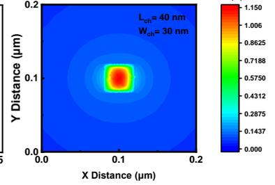
Fig. 15. Simulation result of an  $\text{In}_2\text{O}_3$  GAA nanoribbon FET with  $L_{\text{ch}}$  of 40 nm and  $W_{\text{ch}}$  of 30 nm, showing little temperature increase.
