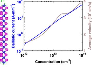
Fig. 19. Ballistic current density and average electron velocity versus carrier density, from DFT simulation of  $\text{In}_2\text{O}_3$  slab.
