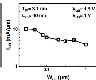
Fig. 10.  $I_{\text{ON}}$  of the  $\text{In}_2\text{O}_3$  GAA nanoribbon FETs under channel width scaling from 1  $\mu\text{m}$  down to 30 nm. Each  $W_{\text{ch}}$  data is from 5-10 devices.
