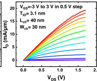
Fig. 17. Pulsed I-V results of output characteristics of an  $\text{In}_2\text{O}_3$  GAA FET, showing maximum  $I_{\text{ON}}$  of 19.3  $\text{mA}/\mu\text{m}$ .
