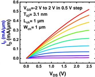
Fig. 5. Output characteristics of a typical  $\text{In}_2\text{O}_3$  GAA nanoribbon FET with  $L_{\text{ch}}$  of 1  $\mu\text{m}$  and  $W_{\text{ch}}$  of 1  $\mu\text{m}$ , showing saturation at large  $V_{\text{DS}}$ .
