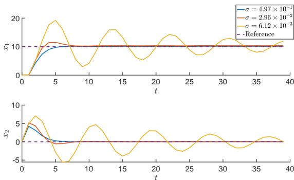
Fig. 1. State trajectories  $x(t) = (x_1(t), x_2(t))$  controlled by solving (13) in a receding horizon fashion for three data sets with varying degrees of persistency of excitation. The legend indicates the minimum singular value of the data matrices (2) used for prediction in (13).
