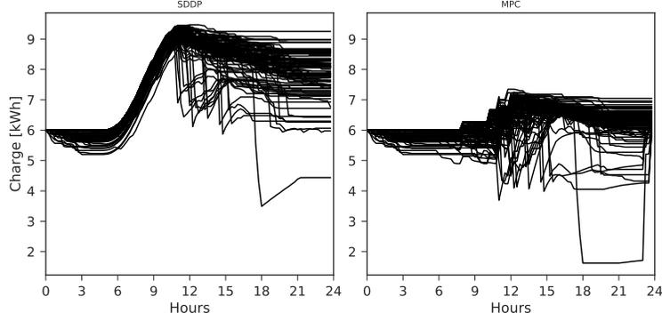
Figure 6: Hot water tank trajectories for SDDP (left) and MPC (right) during Summer day
