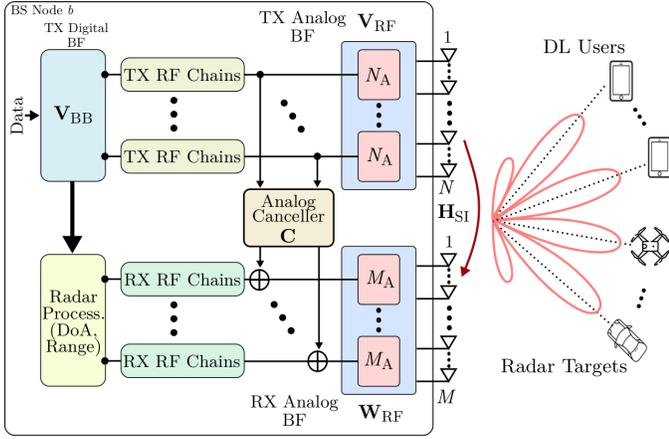
Fig. 1. The considered FD-enabled massive MIMO ISAC system, where the FD hybrid A/D beamforming BS communicates with DL users and simultaneously detects corresponding DoA and range of radar targets.
