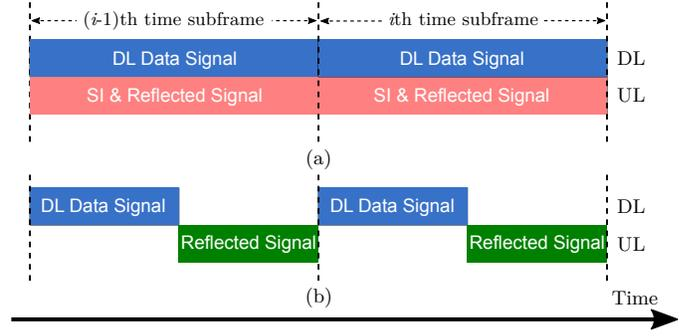
Fig. 2. (a) The Proposed FD-enabled ISAC scheme and (b) the conventional HD-based ISAC signaling in each time subframe.
