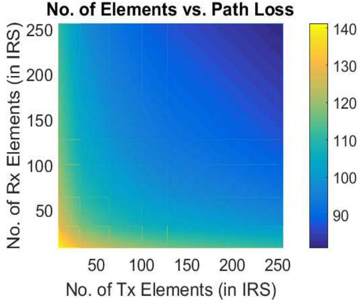
Fig. 6. No. of Tx-Rx elements vs. path loss
