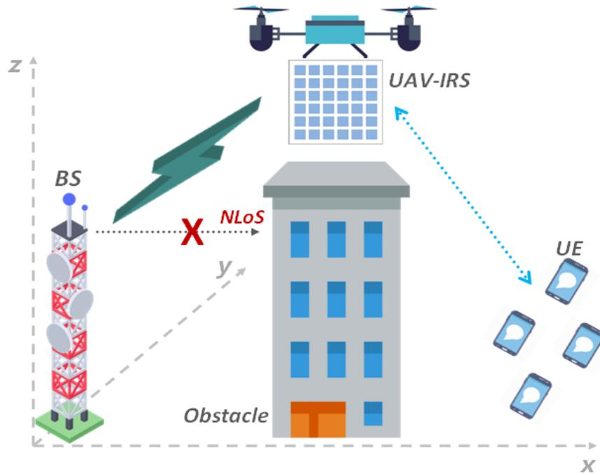
Fig. 1. IRS-empowered UAV-assisted wireless network
