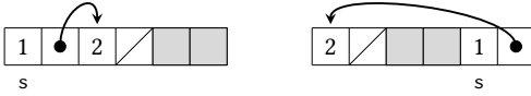
(a) One possible memory representation of s \mapsto [1, 2] . (b) A distinct representation of the same state.
