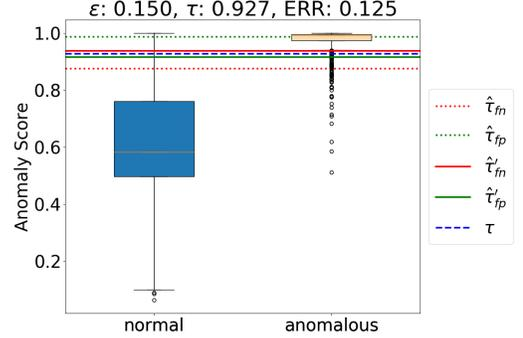
**Figure 3: Box Plot and thresholds on the *celeba* dataset using the DevNet anomaly detector.  $\hat{\tau}_{fp} > \hat{\tau}_{fn}$  holds under the original error constraint ( $\epsilon \leq 0.05$ ). By using Alg. 1,  $\hat{\tau}'_{fn} \geq \hat{\tau}'_{fp}$  under the relaxed error constraint ( $\epsilon \leq 0.15$ ).**
